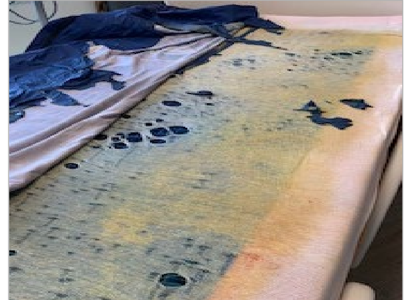
Inside of top mattress cover is DISINTEGRATED BY DISINFECTANT use as well as fire barrier sock protecting the patient.
